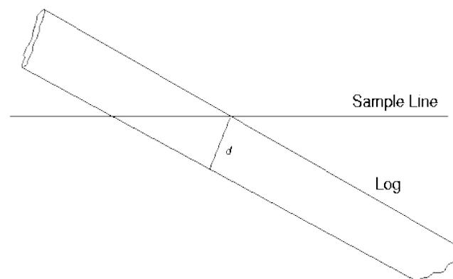
Figure 1. an example of how to measure the down log on the transect
